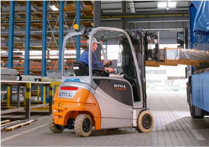
Trucks with Li-ion batteries stand out thanks to higher performance and are also suitable in particular for multi-shift operations. Opportunity charging means batteries no longer need exchanging.
